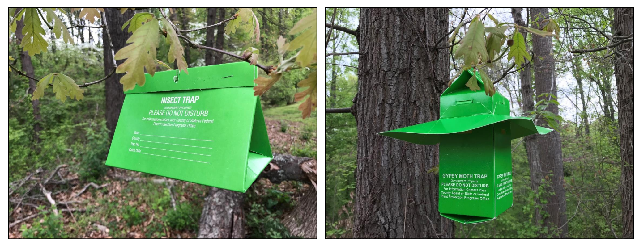
Delta traps are used to monitor low density (<5 moths per trap during a season) gypsy moth populations. Annually, ~60,000 traps are monitored in the STS program area.
