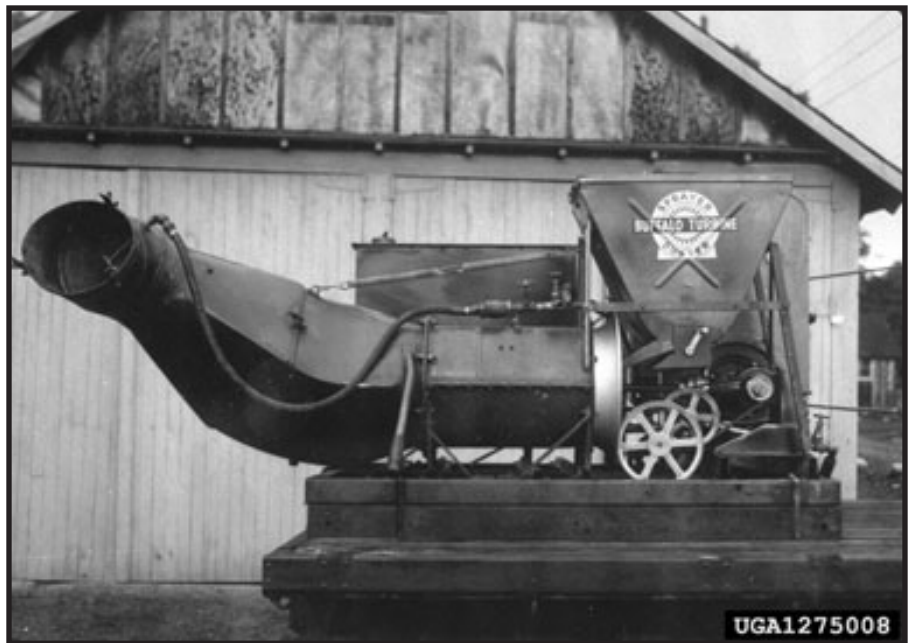
Figure F-1. This insecticide mist blower, designed and constructed in 1946 by Quincy Forestry Department, MA, was used to spray trees in residential areas.
